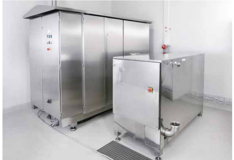
Pipe clearing unit and a lean phase cleaning unit
